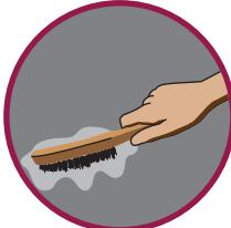
Strip all the old paint and remove all the loose dust, grease, fungus and algae by sanding or wire brushing.
