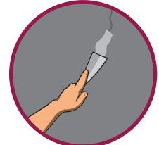
Cracks, holes, dents and damp areas should be repaired properly before painting.
